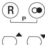
Press the R-key and the redial key at the same time. (The „P“ for „Programming-mode“ appears in the display.)
